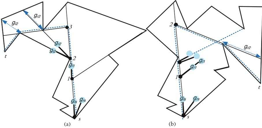
**Fig. 4.** The dotted path is the robot search path from  $s$  to  $t$ . (a) A disappearance event occurs at point 1. At point 2, event (1) arises that updates  $g_l$ , also an event (2) arises that updates  $g_r$  and sets  $g_r$  as an inactive gap. At point 3, the active gap  $g_l$  merges with the inactive gap  $g_r$ . (b) At point 2 the active gap  $g_r$  merges with a non-primitive gap.
