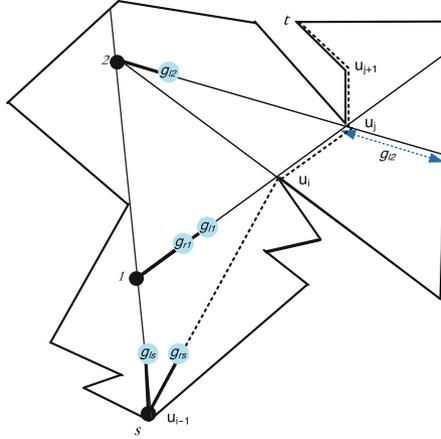
**Fig. 5.** At the start point both of  $g_l$  and  $g_r$  are active. At point 1,  $g_l$  becomes inactive. At point 2,  $g_r$  becomes inactive, as well as  $g_l$ . So, the robot makes a turn at this point. The dotted path is the shortest path from  $s$  to  $t$  and  $u_i u_j$  is an eave.
