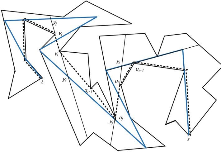
**Fig. 7.** The general case in which shortest path from  $s$  to  $t$  has both left and right turns. Bold path is the robot search path.
