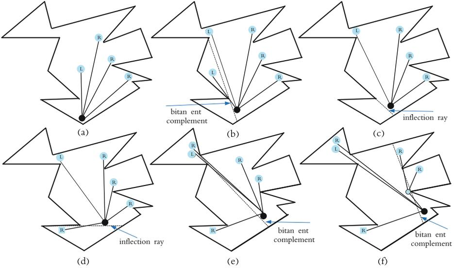
**Fig. 2.** Illustration of the dynamically changes of the gaps as the robot moves towards a gap. The dark circle denotes the location of the robot, and squares and other circles display primitive and non-primitive gaps respectively. (a) Existing gaps at the beginning. (b) A split event. (c) A disappearance event. (d) An appearance event. (e) Another split event. (f) A merge event.
