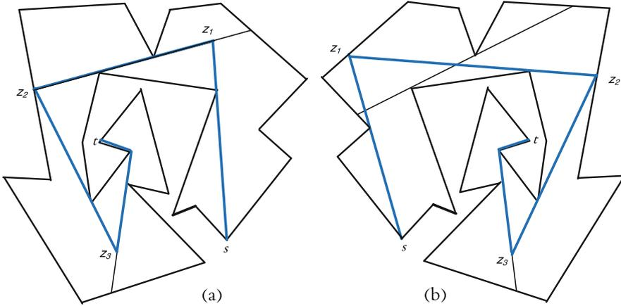
**Fig. 6.** The bold path is the robot search path. The left and right tangent from each turn point  $z_i$  lies inside the street. (a) Shortest path from  $s$  to  $t$  has only left turns. (b) Shortest path from  $s$  to  $t$  has only right turns.
